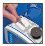
Grasp thumb tab on valve and insert firmly into left pocket. Press down on thumb tab to ensure valve is fully seated. Thumb tab should align with slot in blue door. Blue door will not close if tab is not fully seated.
